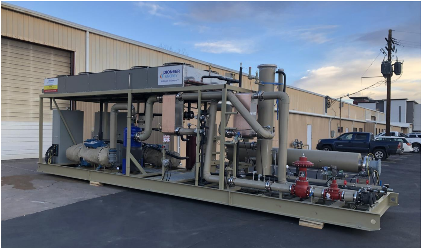
Refrigeration, Separation & NGL Stabilization
